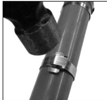
8. Hammer down buckle ears to complete BAND-IT clamp.
