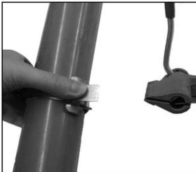
7. Remove tool, holding stub of band down with thumb.
